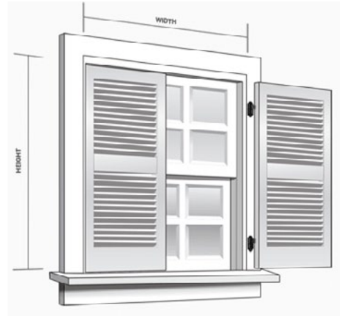
Correct sizing of a shutter
