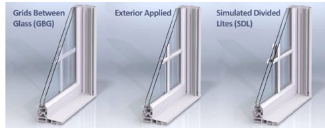
Illustrating the difference between GBG and SDL window design
